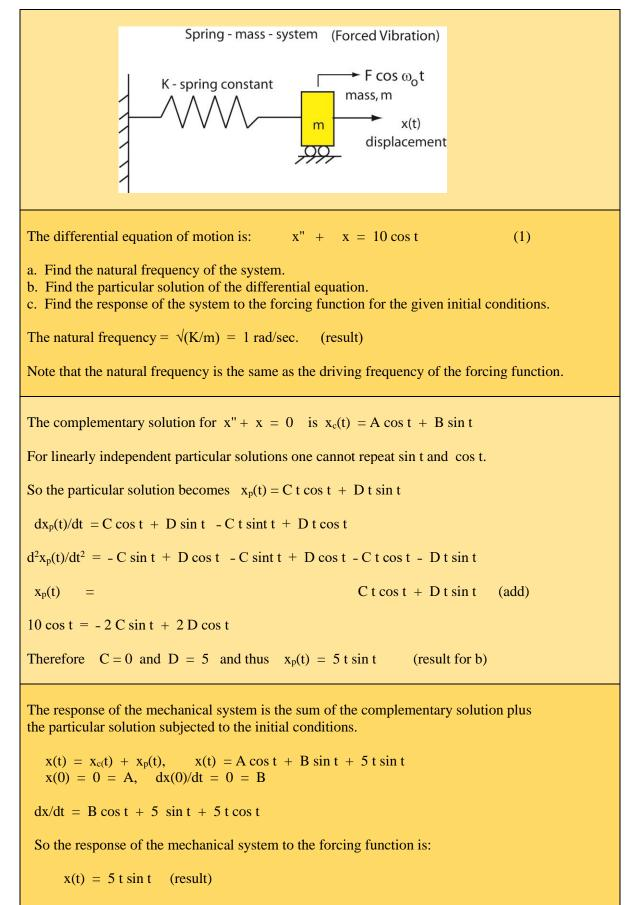
Note: The amplitude of response increases with time.
