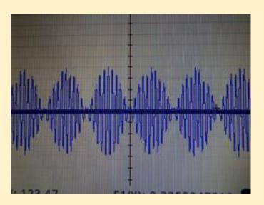
The "envelope" is governed by  $\sin(0.05t)$  with a period of  $40\pi$  seconds and shows the beats (or modulation). The "High Frequency" vibration within the "envelope" is governed by  $\sin(1.05t)$  with a period of  $1.9\pi$  seconds.
