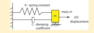
The differential equation is:  $d^2x/dt^2 + (C/m) dx/dt + (k/m) x = 0$ with initial conditions x(0) = 9/100 m and dx(0)/dt = 0 m/sec.
