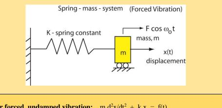
**For forced, undamped vibration:**  $m d^2x/dt^2 + k x = f(t)$
