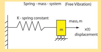
The differential equation for free, undamped vibrations is:
