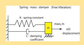
The differential equation for free vibrations with damping is:
