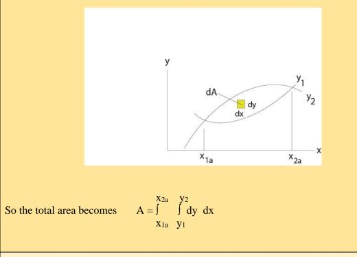
Here the first integration is on the y-variable. You can picture this as "sweeping" the element of area from  $y_1$  to  $y_2$  followed by "sweeping" the rectangle from  $x_{1a}$  to  $x_{2a}$ .
