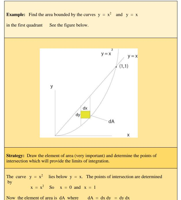
For the element shown above, choose to integrate on the variable y first. i.e. Sweep in the "y-direction first. So dA = dy dx and the integral becomes:
