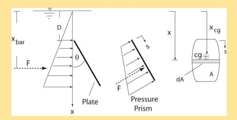
The elemental pressure force dF acting on the element of area dA is dF = PdA. Now the pressure, P, varies linearly with depth, x. So  $P = \gamma x$  and the differential pressure force is  $dF = \gamma x dA$ . So integration gives the total hydrostatic pressure force, F.
